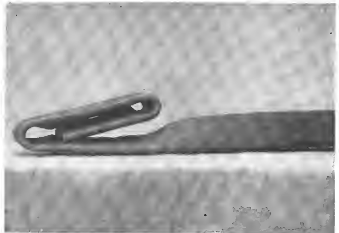
FIG. 2.—C-46-O Krupp chassis frame steel deformed to show extent of bending without showing cracks. Under a compression test this steel showed set when subjected to 85,296 pounds per square inch.
